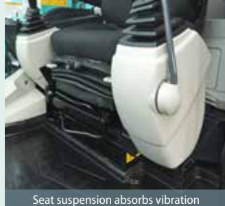
Seat suspension absorbs vibration
