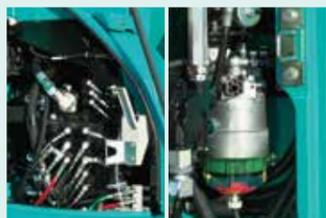
Control valve/water separator tank/air cleaner
