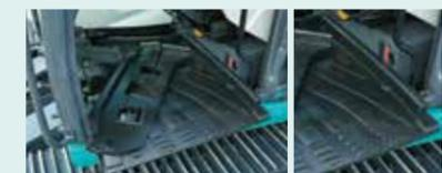
Detachable two-piece floor mat has handles for easy removal. The mat's raised edges trap dirt and grit for easy cleaning.
