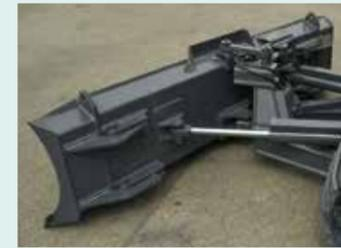
The 6-way dozer blade has Power, Angle and Tilt capability (PAT) operated from the cab. With a single control lever, the blade can be angled 25 degrees to the left or right for dispensing earth and materials away from the operator's path. The blade also tilts up on the left and right sides by 455 mm for slope grading, culverts and ditches.
